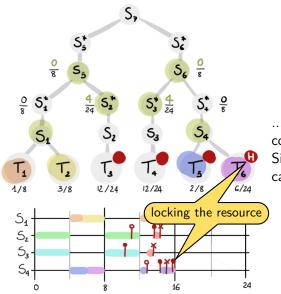
$\dots T_5$  uses the resource and completes before its deadline. Since the resource is free,  $T_6$  can lock it.
