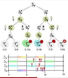
...since  $T_3$  and  $T_4$  already used and released the resource, it's just normal execution and budget consumption.
