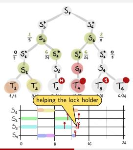
$T_5$  does not spin because the lock holder *is not already executing*, but it lets execute  $T_4$
