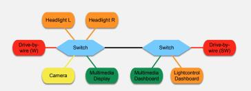
RT-Ethernet Residual Bus Simulation
