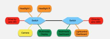
RT-Ethernet Residual Bus Simulation
